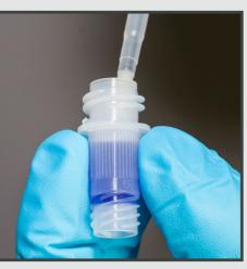
> Transfer the sample slowly into the heating tube. Slowly rinse the tip once to remove the sputum.
