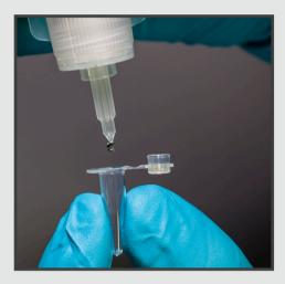
> Extract 30 µl of the DNA directly into the reaction tube by squeezing the adsorbent tube.
