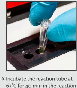
unit. The reaction is automatically inactivated by a further incubation step at 80°C for 5 min.
