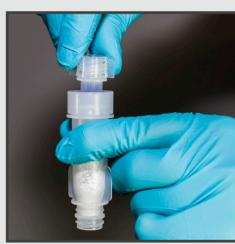
> Screw the heating tube onto the adsorbent tube.
