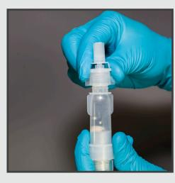
> Screw the injection cap onto the other side of the adsorbent tube.
