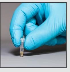
> Flick down the reaction tube until the reaction mixture is collected at the bottom.
