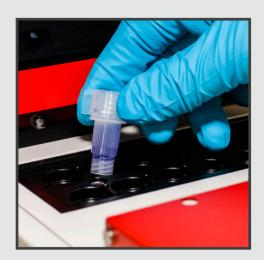
> Incubate the tube in the HumaLoop T heating unit at 90°C for 5 min.
