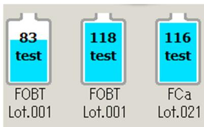
For the R1 and R2 reagents, the remaining volume is displayed with bottle graphics. In addition, the test item, lot number, and available test count are displayed.
