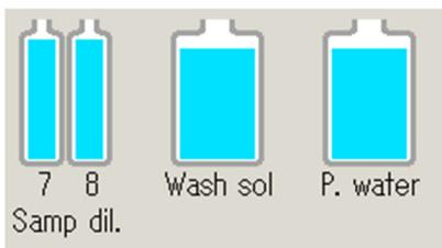
For the diluent, washing solution, and purified water, the remaining volumes are displayed using a bottle graphic.
