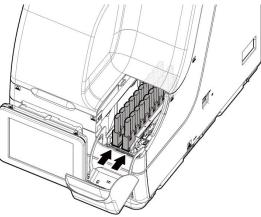
2 Set the rack into the rack lane with rack position No.1 at the innermost end. Pay close attention to set the rack properly.
