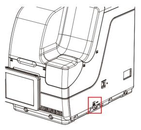
2 Check that the hose is connected to the drain connect or at the right side of the system.
