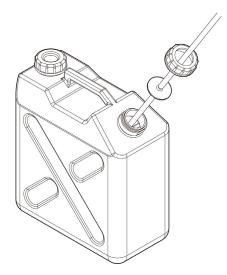
1 Connect the hose to the drain tank.
