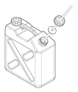
1 Remove the hose from the drain tank.
