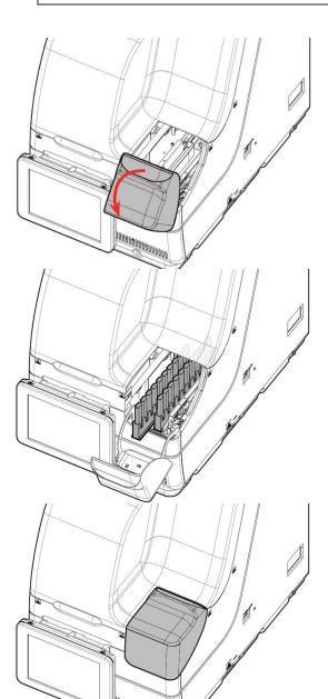
2 Remove the racks which testing is finished.
