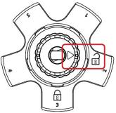
6 Remove the used cell and replace it.
