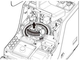
5 Remove the cell retainer.
