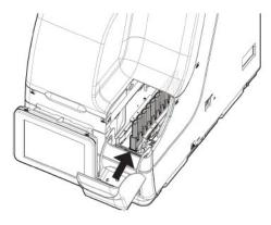
Remove the rack from the rack lane for which the lane information is "Replace" or "Waiting."
