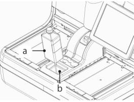
1 Set the buffer bottle (a) to the buffer compartment (b).
