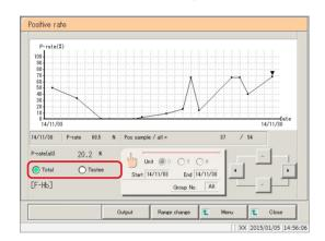
Select the display mode for positive samples (by Total/Testee).
