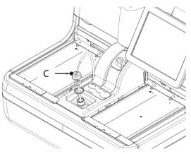
Remove the cap of the buffer bottle, and insert the hose (c).
