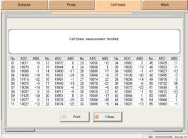
When cell blank measurement is complete, touch the  $\{Close\}$  button.
