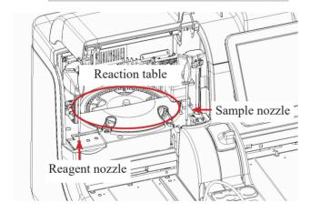
If the sample nozzle and reagent nozzle are on the reaction table, move them by hand so as to not hinder work.
