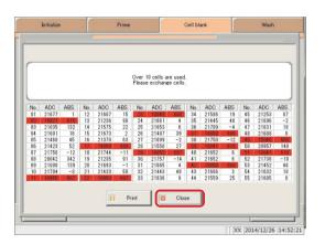
1 Measurement cells that cannot be used are shown in red.
