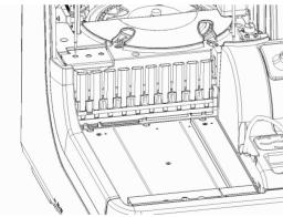
4 Latch the "STAT rack position" conveyance bar into the groove in the middle of the rack, and place the rack.
