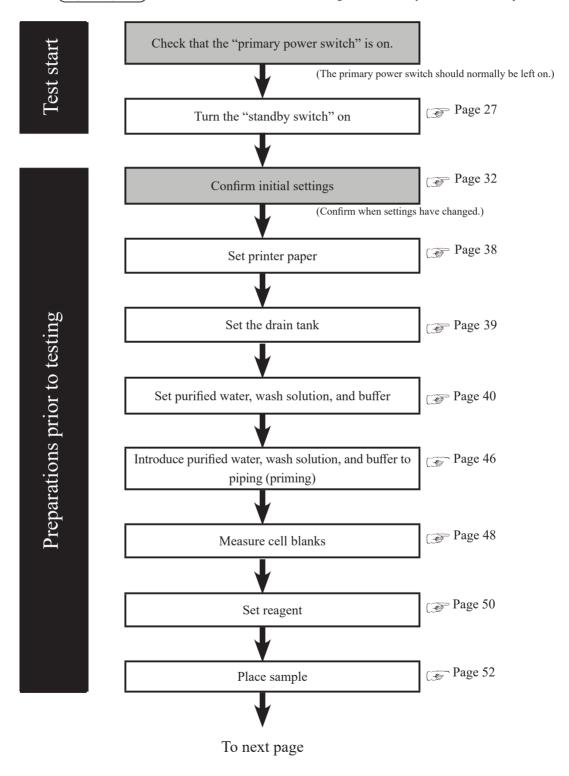
Explanatory note : If "Cell blank" is checked in "Auto start" in close mode, cell blank measurement will be automatically run when the system starts.
