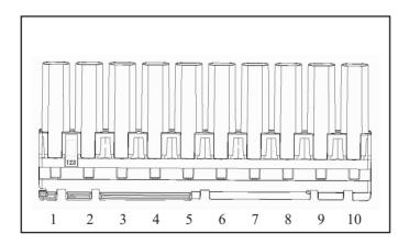
Explanatory note: The numbers in the diagram indicate the rack position number. They are numbered from left (No. 1) to right.
