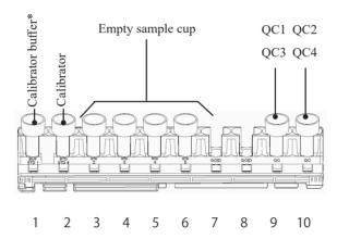
Explanatory note : In the case of the hemoglobin, QC samples can be ID-managed by erection of containers with QCID (bar code for QC) attached to positions No. 7 and No. 8 in the rack.
