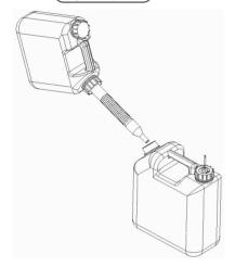
Add purified water to the purified water tank.
