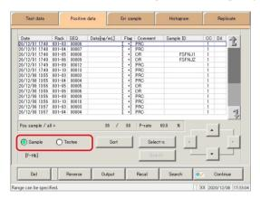
Select the display mode for positive samples (by sample/testee).
