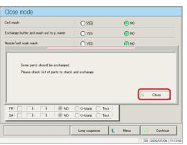
2 If there are parts for which the exchange period has been exceeded, "Some parts should be exchanged. Please check list of parts to check and exchange." is displayed.
