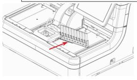
Set the rack to the rack supply unit with rack position No. 1 on the left side.
