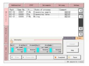
The images of the reagent bottle and buffer bottle show how much reagent is left in the bottles.
