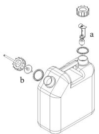
Attach a maximum-level sensor (a) and hose (b) to each drain tank port (two).
