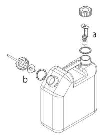
Attach a maximum-level sensor (a) and hose (b) to each drain tank port (two).
