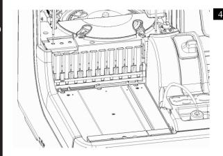
Latch the "STAT rack position" conveyance bar into the groove in the middle of the rack, and place the rack.
