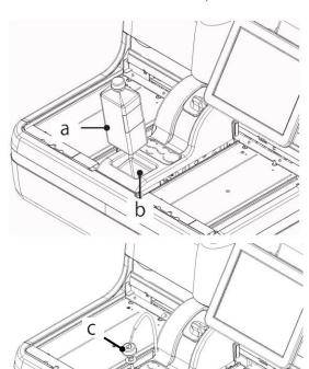
Set the buffer bottle (a) to the buffer compartment (b).
