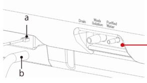
Confirm that the zero-level sensor (a) and hose (b) are connected to "Purified Water" at the "installation location for tanks" on the left side of the system.
