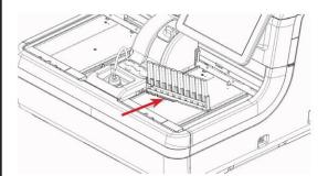
Set the rack to the rack supply unit with rack position No. 1 on the left side.
