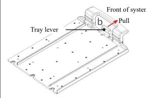
Front of system Pull the tray lever (b) to the front.
