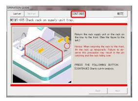
Check the rack supply unit and the rack on the tray.
