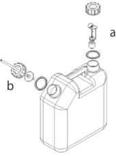
Attach a zero-level sensor (a) and hose (b) to each purified water tank port (two).
