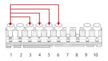
Dispense No. 1 calibrator buffer to the sample cups in rack position numbers 3 through 6.
