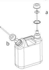
Attach a zero-level sensor (a) and hose (b) to each wash solution tank port (two).
