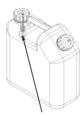
Zero-level sensor Maximum-level sensor
